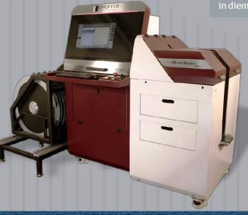
With an operator it is possible to produce the cutting lines through a machine and the creasing lines through an other machine simultaneously.
