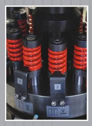
The Bendmaster can process the 2pt. - 3pt. - 4pt. steel coils up to 30 mm height without needing a change the tools at everytime by a carousel tool unit in which 12 different tools are integrated.
