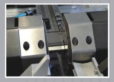
Extreme compact bending head with 2 driving motors which are working simultaneously. Exchange time of the bending heads is under 1 minute.
