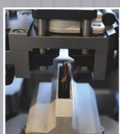
Trim-cut tool is also working with a servo linear actuator, by cutting from the up and down side through the geometry of bended parts. There is the possibility to cut creasing rules directly on the trim-cut unit to achieve a higher production speed.
